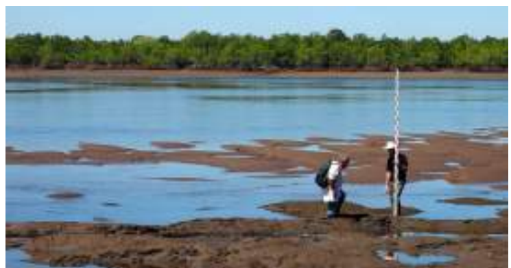
Figure 3: Researchers assessing the high and low tide points at a restoration site. It is important to understand the elevation of a restoration site relative to sea level as mangroves grown in the top half or top third of the intertidal zone only. Working too low down within the intertidal zone (below mean sea level) will result in poor results or project failure.
