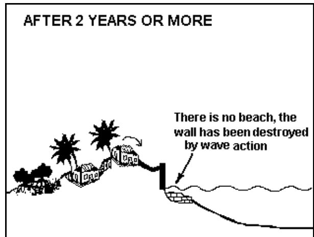
Figure 7: Over time, more erosion removes the last of the beach, and the wall collapses
